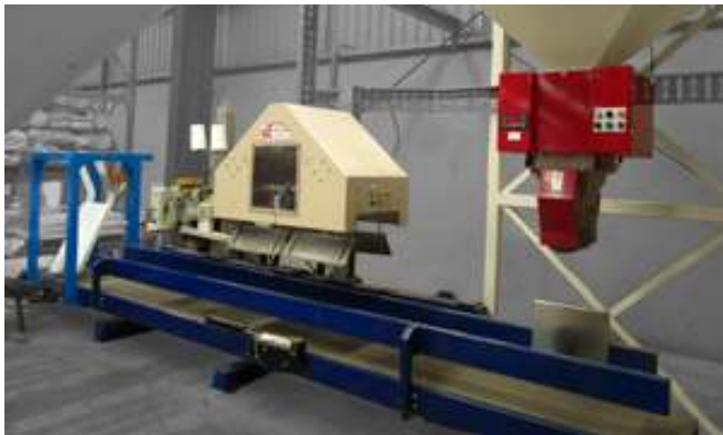
Bagging line application filling woven poly and laminated woven poly bags with various free flowing products
