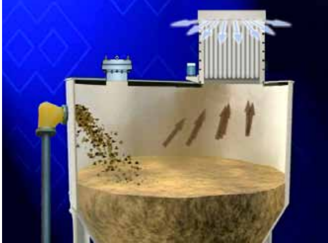
Dust is separated from the dirty air flow while clean air is evacuated from the filter
