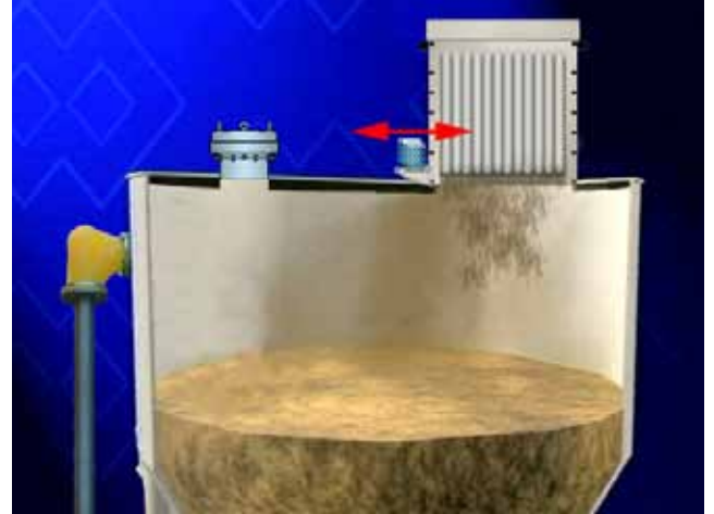
Dust drops down into the silo due to shaking filter elements
